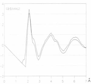
Fig. 2. Experimental and RMC simulated total reduced radial distribution functions of glassy  $Ni_2B$ . (1)  $Ni^{58}$ ; (2)  $Ni^{62}$ ; (3)  $Ni^{0}$ . Again, the curves from the simulation are above those measured.
